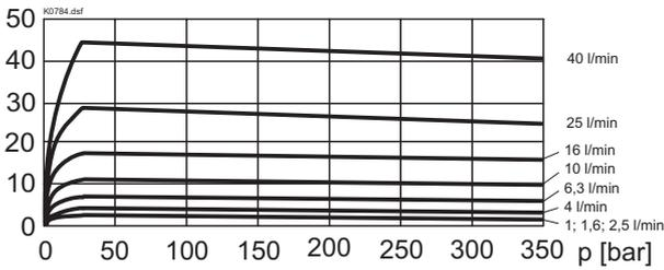
$\Delta p = f(Q)$  Pressure drop characteristics for return flow (from 2  $\rightarrow$  1)
