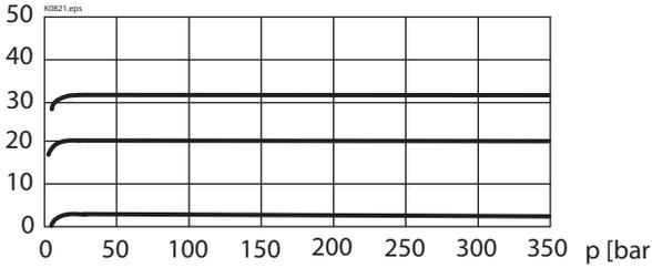
$Q = f(n)$  Volume flow adjustment characteristic ( $p = 350 \text{ bar}$ )
