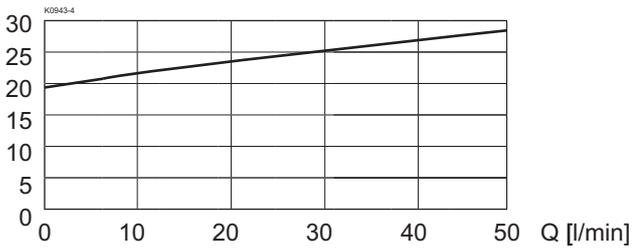
$\Delta p = f(Q)$  Pressure drop-volume flow characteristic  $1 \rightarrow 3$
