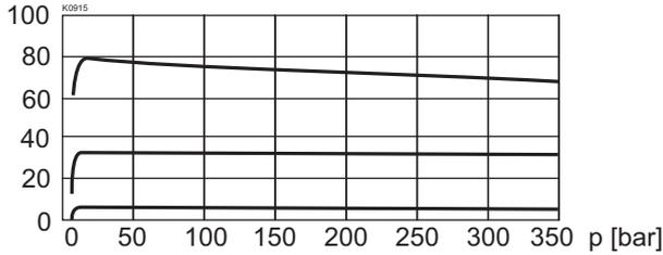
$Q_L = f(p)$  Leakage volume flow characteristic
