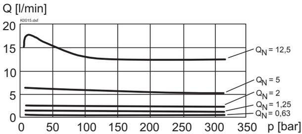
$\Delta p = f(Q)$  Pressure drop characteristics for return flow (from 2 → 1)
