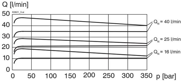
$Q = f(n)$  Volume flow adjustment characteristic ( $p = 350 \text{ bar}$ )
