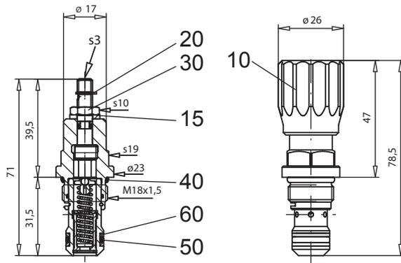
Cavity drawing according to ISO 7789-18-01-0-98
