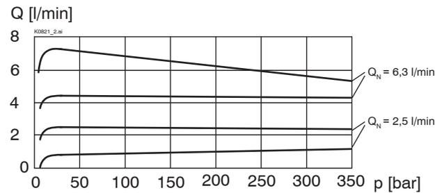
$Q_L = f(p)$  Leakage volume flow characteristic
