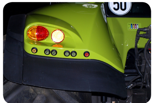
M30 push buttons at the back of a tractor for controlling a rear hoist unit
