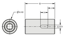
Part number example: GSC25x0500 = glide screw assembly, cylindrical nut, 0.250 inch diameter by 0.500 inch lead
