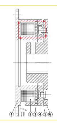
Depending on the size of the clutch or brake, the installation must provide for an air gap of between 0.2 and 0.5 mm between the drive hub and the armature disc. The purpose of this air gap is to ensure complete separation of the input and output drives when no current is applied.
