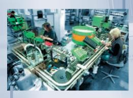
Assembly and testing of pressure switches on partially or fully automated plant.
