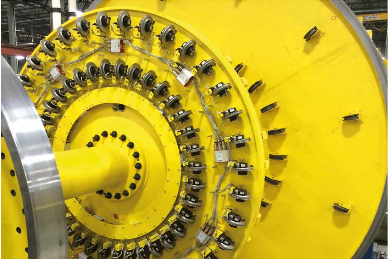
RTM X42 | Application in Cage Type Stranding Machine
