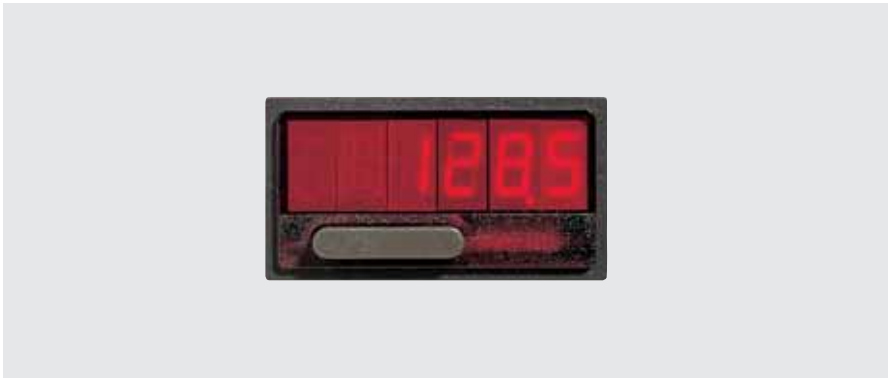
Remote counter To display the charge value. The remote counter can be installed up to about 400 m away from the Scale Processor. Reset of the remote counter is possible at the remote counter itself. Optional built in a housing.
