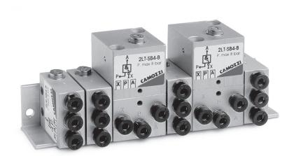
Basic logic functions Series 2L are available in 5 different models and can be mounted separately by means of 2 passing holes in the body. Bracket Mod. 2LQ-8A allows to have the inlets and outlets on the front side, facilitating the mounting of the connection tubes.
