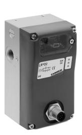
Series LRWD2 and LRPD2 digital proportional servo valves are direct driven 3/3-way valves with a patented rotating spool system with closed loop control circuit. The electronic board is integrated into the valve's body ready to connect.
