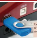
Easy transfer of measuring data or device configurations between measuring systems and PCs.
