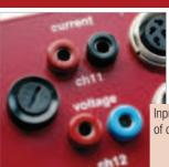
Input yescks for the direct measuring of current and voltage.
