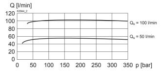
$\Delta p = f(Q)$  Pressure drop volume flow characteristic  $1 \rightarrow 3$
