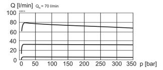
Q<sub>1</sub> = f (p) Leakage volume flow characteristic
