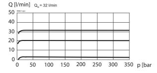
Q = f (n) Volume flow adjustment characteristic (p = 350 bar)
