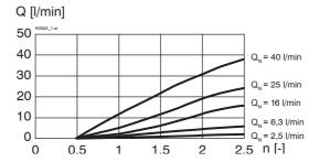
Q<sub>i</sub> = f (p) Leakage volume flow characteristic
