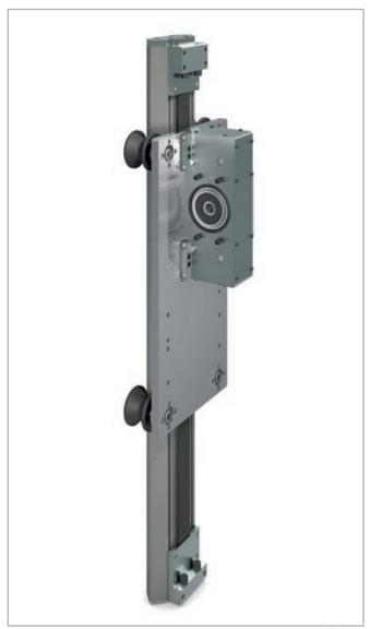
ZSY products are self-supporting extruded aluminum actuators driven by a polyurethane belt system. Due to their deep hard anodized surface treatment and their plastic compound coated rollers, ZSY series can achieve exceptionally high performances and load capacity with no maintenance or lubrication required. They also provide total reliability even in dirty environments, with uniquely quiet operation.
