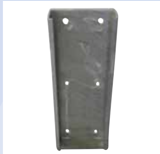
Back plate. Galvanized 770 x 270 x 80 mm Weight: 26 kg Remember rubber spacer
