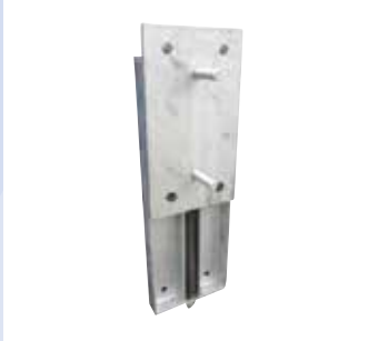
Back plate for 450 mm buffer 720 x 250 x 66 mm Weight: 32 kg Spring loaded. Follows the truck when loading.
