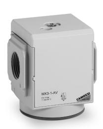
These soft start valves allow a gradual increase of the pressure in pneumatic systems. The pressure increases slowly according to the set regulation until it reaches half of the set value, then it increases rapidly. The valve poppet shifts slowly and securely to the open position to prevent sudden and unsafe movements of the pneumatic components in the system.
