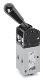
The manual valves Series 3 (G1/8) and Series 4 (G1/4), 3/2 - 5/2-way and 5/3-way, are available with devices designed to satisfy different needs. The 3/2-way valves Series 3 and 4 are normally closed when 1 is the inlet; they can also be normally open when 3 is the inlet.
