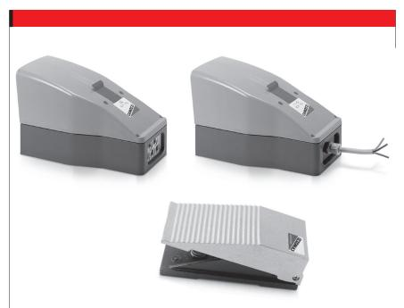
The pedals can be supplied in either a pneumatic or electrical foot operated version. The pneumatic type is available with a 5/2 valve and G1/4 front ports, which allow the fittings and silencers to be assembled conveniently on the front face. A 3/2 operation can be obtained by closing an outlet port. The electrical type is available with
