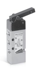
In order to facilitate the use of limit switch valves in applications where very low actuating forces and high flow rates are required, the Series 3 and Series 4 valves are equipped with new mechanical devices designed for this purpose. The Series 3 valve is designed with a mechanical lever which when operated releases an internal pilot signal to atmosphere. The sensitivity can be increased by adding a "whisker" or rod of Ø 3 mm to the lever.
