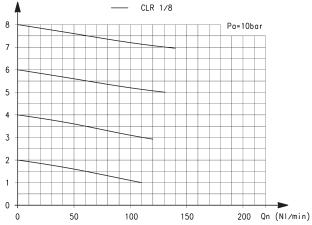
Pa = Inlet pressure - Pr = Regulated pressure Q = Flow CLR 1/4-6 6 bar  $\Delta$ P1 = 209 NI/min CLR 1/4-8 6 bar  $\Delta$ P1 = 310 NI/min
