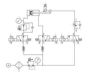
For a correct use of the rod lock Mod. RLC a pneumatic connection is recommended (as shown in the examples).
