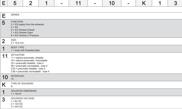
Pneumatically actuated valve, monostable - size 10,5
