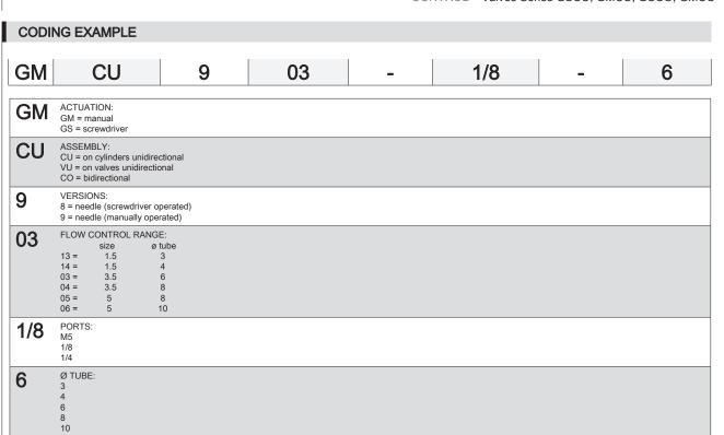
To ensure the right choice of unidirectional flow controller, proceed as follows: calculate the quantity of air in NI/min (see cylinder Table); determine the stroke time of the cylinder; refer to graph to see which controller is the right type.
