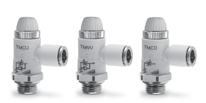
The unidirectional and bidirectional flow controllers, series TMCU, TMVU, TMCO have been revised in order to decrease their dimensions and improve their flow rate characteristics. Their construction allows for easy assembly to cylinders and valves and allows the regulation adjustment to be precise and gradual.
