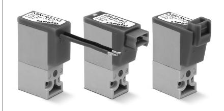
Series K directly operated solenoid valves are available as 3/2-way either NC or NO versions. Both versions can be mounted on single sub-bases or manifolds and they are equipped with a manual override which makes the plants setting easier.
