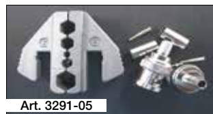
Art. 3291-05 Coaxial RG 58.59.62.6. 6.48 / 5.41 / 2.5 / 1.72 / 8.23 mm 2 0.255 / 0.213 / 0.1 / 0.68 / 0.324"
