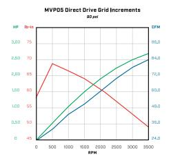
Example of the MVPO5 direct-drive air motor performance curve. See individual catalog pages for model-specific performance data.
