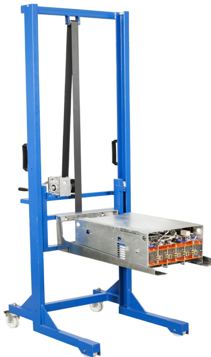
Figure 6.5: Power arm insertion/extraction/movement trolley
