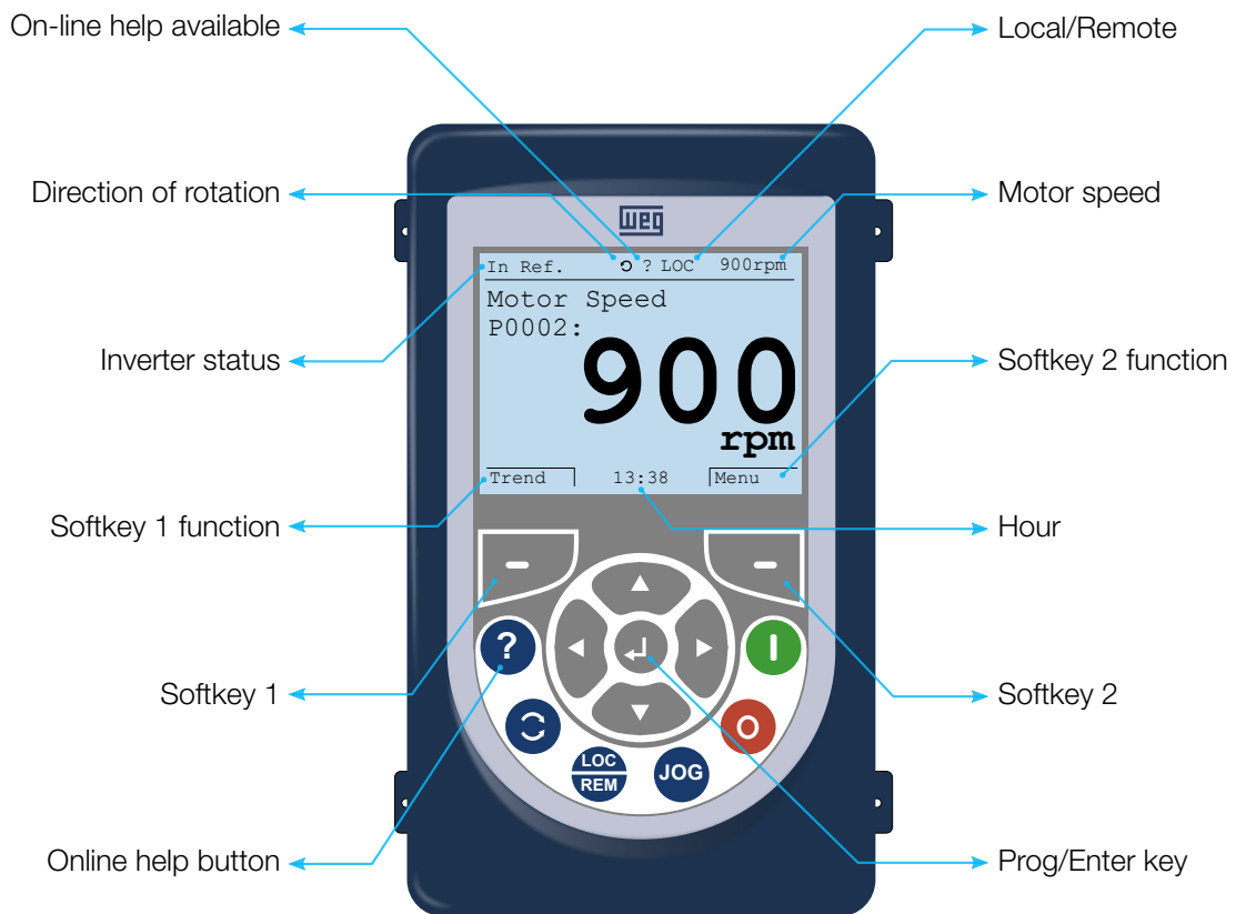
Figure 4.1: MVW3000 inverter HMI
