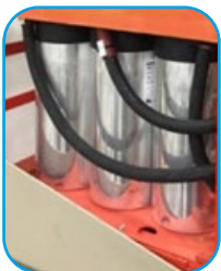
Long life plastic film capacitors for DC link voltage source manufactured by WEG (same capacitors used by the aero-space industry in satellites)
