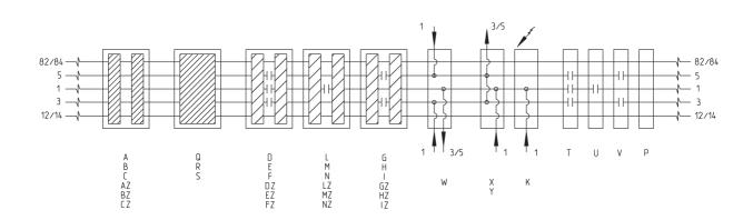
[\*] The subbases A, B, C, D, E, F, G, H, I, L, M, N are available also with a board to be used with monostable solenoid valves. To order this version it is necessary to add Z at the end of the code of the standard subbase. Example: AZ instead of A. For further details we suggest you to see the coding example.
