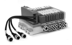
The Multipole version can be connected in a quick and secure way thanks to the electrical connection by means of a pre-wired cable with 25 or 37 pins with in-line or angular connection. It is possible to create zones with differentiated power supply and with separate pressure/exhaust. Thanks to the subbases with monostable board, islands can be realized up to maximum of 24 coils on 20 valve positions with the 25 pin connection and 32 coils on 28 valve positions with the 37 pin connection.
