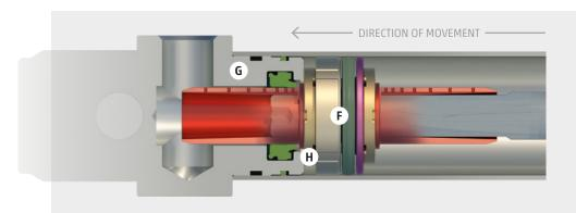
The movement stops when the end stroke position is reached and the piston (F) touches the end cap (G). The presence of a damper (H) absorbs any residual kinetic energy and minimises the impact so that there is no vibration or noise.
