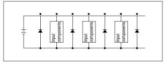
When components are connected with connectors, if a connector is dislocated during energizing, the output circuit could be damaged because of the reason above. Turn off the power before dislocating a connector.
