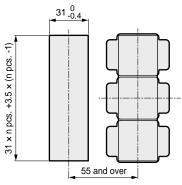
(Note 1): Panel thickness must be 0.5 to 6mm.
