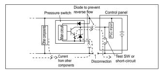
Take countermeasures as followings to prevent damages caused by reverse current.
