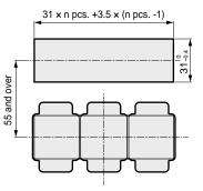
(Note 1): Panel thickness must be 0.5 to 6mm.
