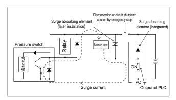
Take countermeasures as followings to prevent damage caused by surge current leading.
