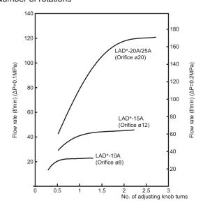
Note1: Set the adjusting dial as follows: for connection port 10A, open a 1/4 turn or more from the fully closed position; for all other port sizes, open more than a 1/2 turn. Using the product with a smaller opening than recommended may cause vibration or fluctuation in flow depending on the working conditions.
