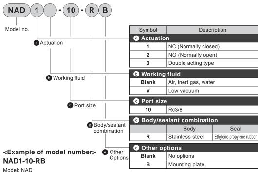
aActuation : NC (Normally closed)bWorking fluid : Air, inert gas, water
