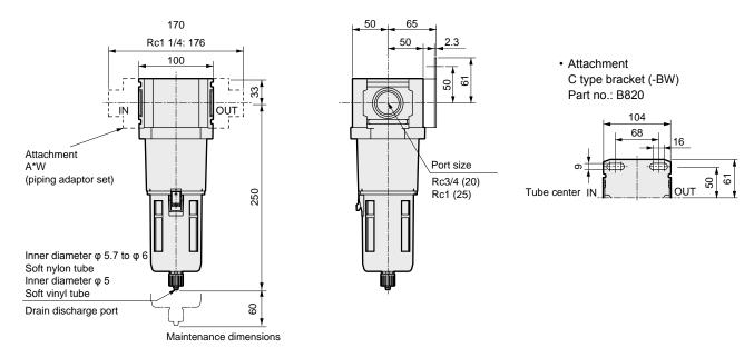
• For the plastic bowl, the dimensions are the same regardless of whether the manual cock or with automatic drain.
