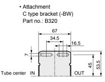
• For the plastic bowl, the dimensions are the same regardless of whether the manual cock or with automatic drain.
