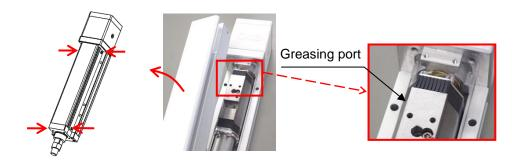
**4** Perform a break-in operation to apply grease.
