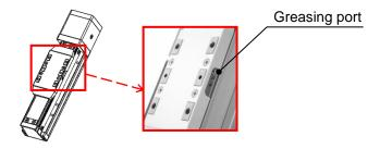
**3** Perform a break-in operation to apply grease.
