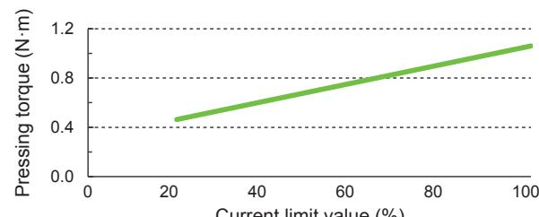
\*1 The pressing torque and current limit value are merely guidelines. Individual motor differences and variations in mechanical efficiency may result in differing actual values, even at the same current value.
