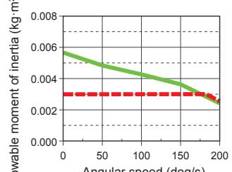
\* When angular acceleration/deceleration is greater than 1700deg/s<sup>2</sup>, operate below the dashed line.
