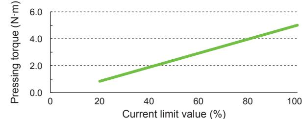
\*1 The pressing torque and current limit value are merely guidelines. Individual motor differences and variations in mechanical efficiency may result in differing actual values, even at the same current value.
