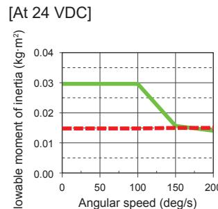
\* When angular acceleration/deceleration is greater than 1700deg/s<sup>2</sup>, operate below the dashed line.
