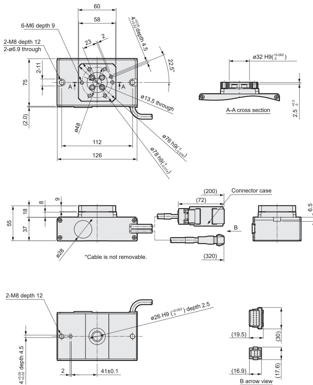
\*1 The origin position of the actuator may differ from the position shown in the dimensions. The origin offset function allows origin setting at any position.
