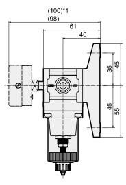
\*1. Dimensions when the digital pressure sensor is assembled.
