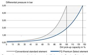
Permanently more capacity plus longer service life: innovative Premium Select element with 30% increase in dirt pick.-up capacity, lower differential pressure and optimised differential pressure curve – for reduced energy consumption.
